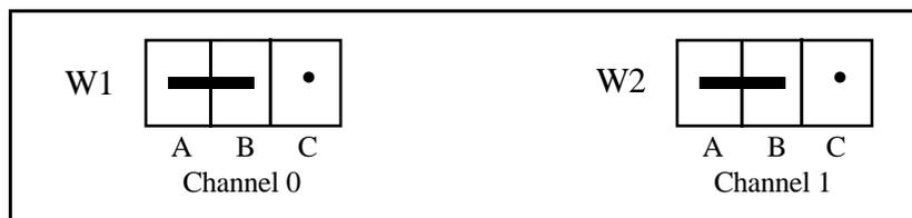
Figure 2-4. DC-Coupled Output Jumper Configuration
