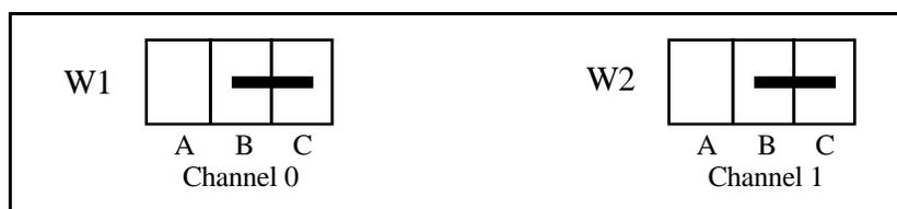
Figure 2-3. AC-Coupled Output Jumper Configuration
